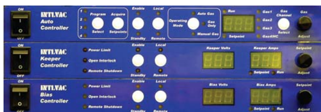
eHC Power Supply Controller
